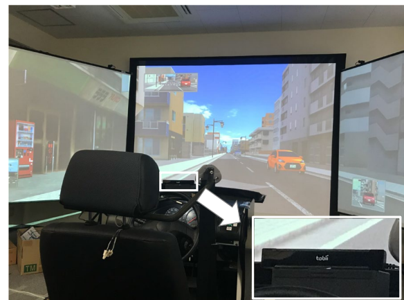
Fig. 1 Experimental setup showing the main view with an inset detail of the eye tracker in the lower right corner
