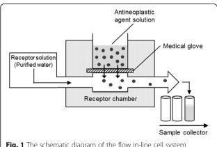
Fig. 1 The schematic diagram of the flow in-line cell system
