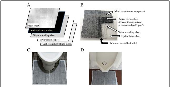
**Fig. 1** HD safe sheet-U (**a**: structure, **b**: photograph) and HD safe sheet-U application in lavatories (**c**: Western style toilet, **d**: Urinal toilet). Presents (**a**) structure and (**b**) photograph of HD safe sheet-U; (**c**, **d**) application of the sheet in lavatories. HD safe sheet-U consisted a nonwoven, adsorption layer that included active carbon at a density of 25 g/m², a water (urine) absorption layer, an opacity film, and a back-side adhesive tape from the top
